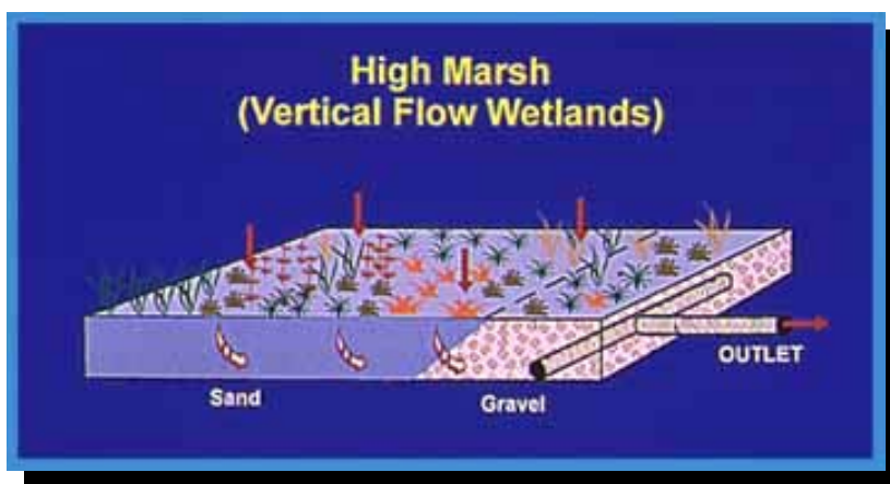
Figure 5-20 Vertical Flow Wetland
