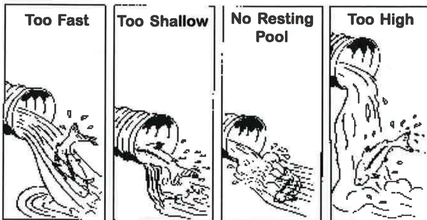
Figure 2.2b Poorly designed or installed culverts with “fish barriers” that prevent fish passage. (Redrawn from Evans and Johnston 1980)
