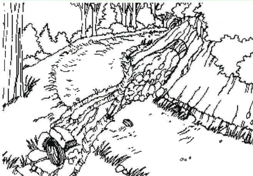
Figure 4.4 Road maintenance is needed to maintain roadway surface drainage patterns and remove slides that block ditches and culvert inlets.
