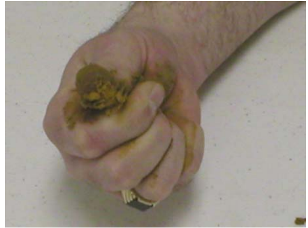
D – Loamy Sand does not form a ribbon
