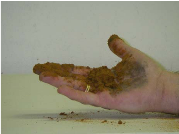
C – Sand does not remain in a ball when squeezed
