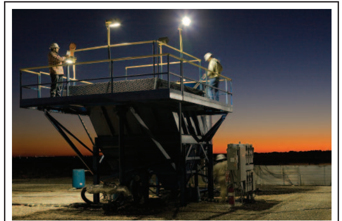
Shown here is one of Devon Energy’s water recycling stations in the Barnett Shale. The machinery includes the first stage of the recycling process, where flocculent is added to make the fine particles congeal. The congealed matter settles to the bottom, making it easier to remove solids from the water.
