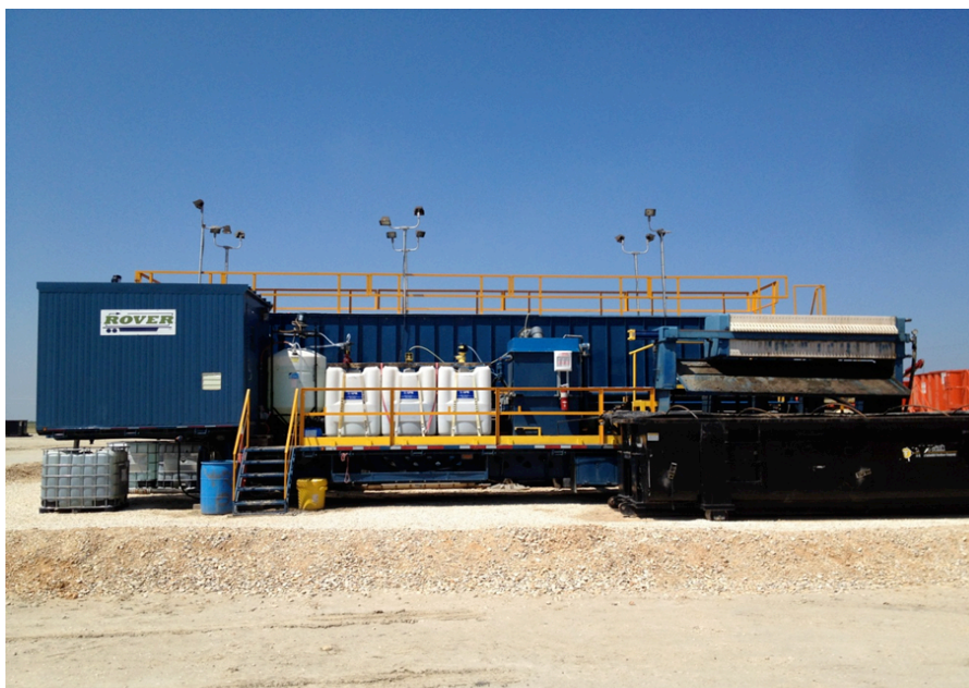
FIGURE 5.0: Fountain Quail's ROVER Mobile Clarification System
