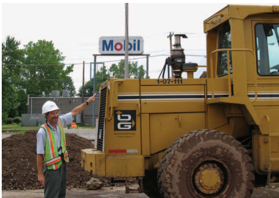
Construction equipment retrofit with a diesel oxidation catalyst.
