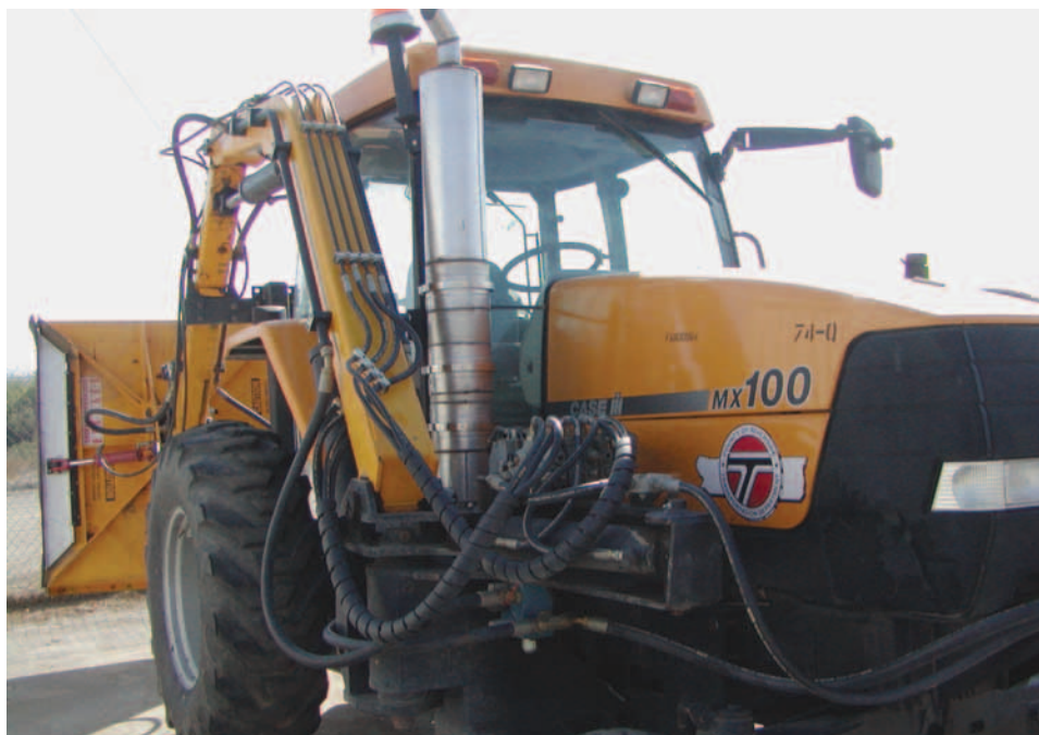
Construction equipment retrofit with a diesel particulate filter.
