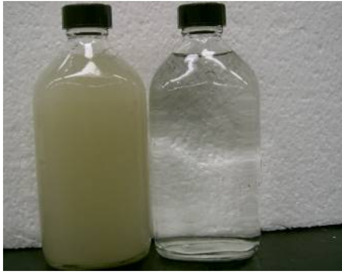
Figure 11. Feed sample (left) and permeate samples (right) of ceramic tubular membrane, 0.005 micron and hollow fibre membrane 0.04 micron of lab prepared mud.
