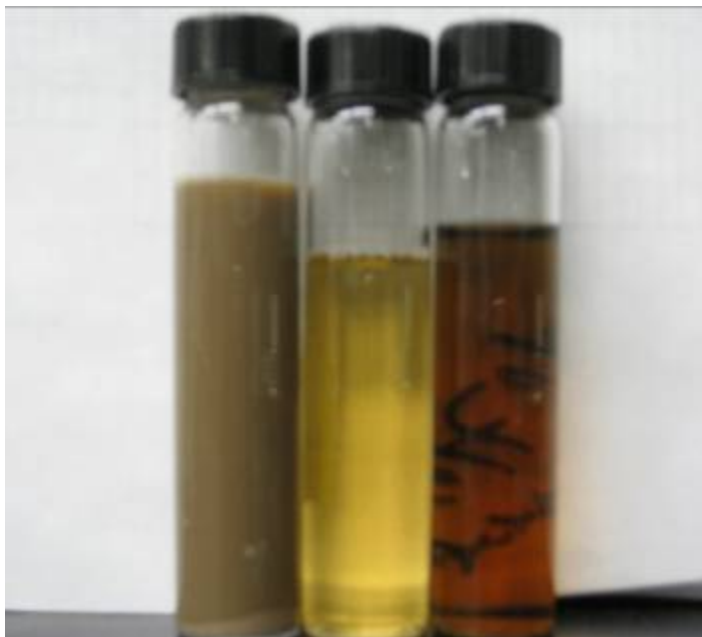
Figure 8. Feed sample (left) and permeate samples, ceramic tubular membrane, 0.005 micron (middle), hollow fibre membrane 0.04 micron (right) of field supplied lignosulphite WBM.
