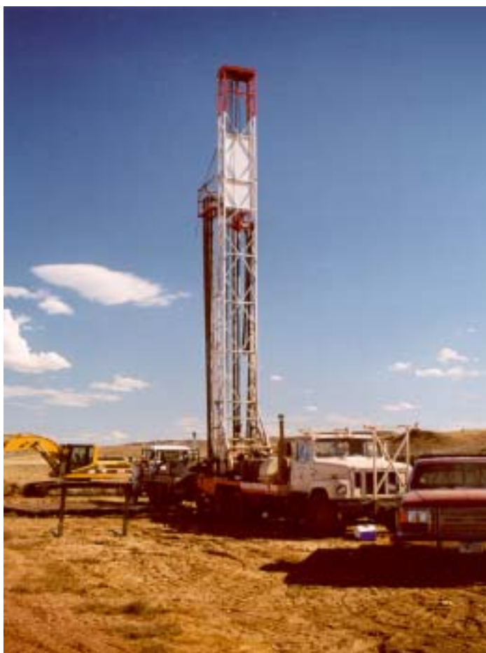
Typical truck mounted drill rig used for shallow CBM wells
