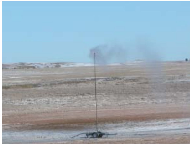
CBM produced water being aerated in the Powder River Basin, Wyoming
